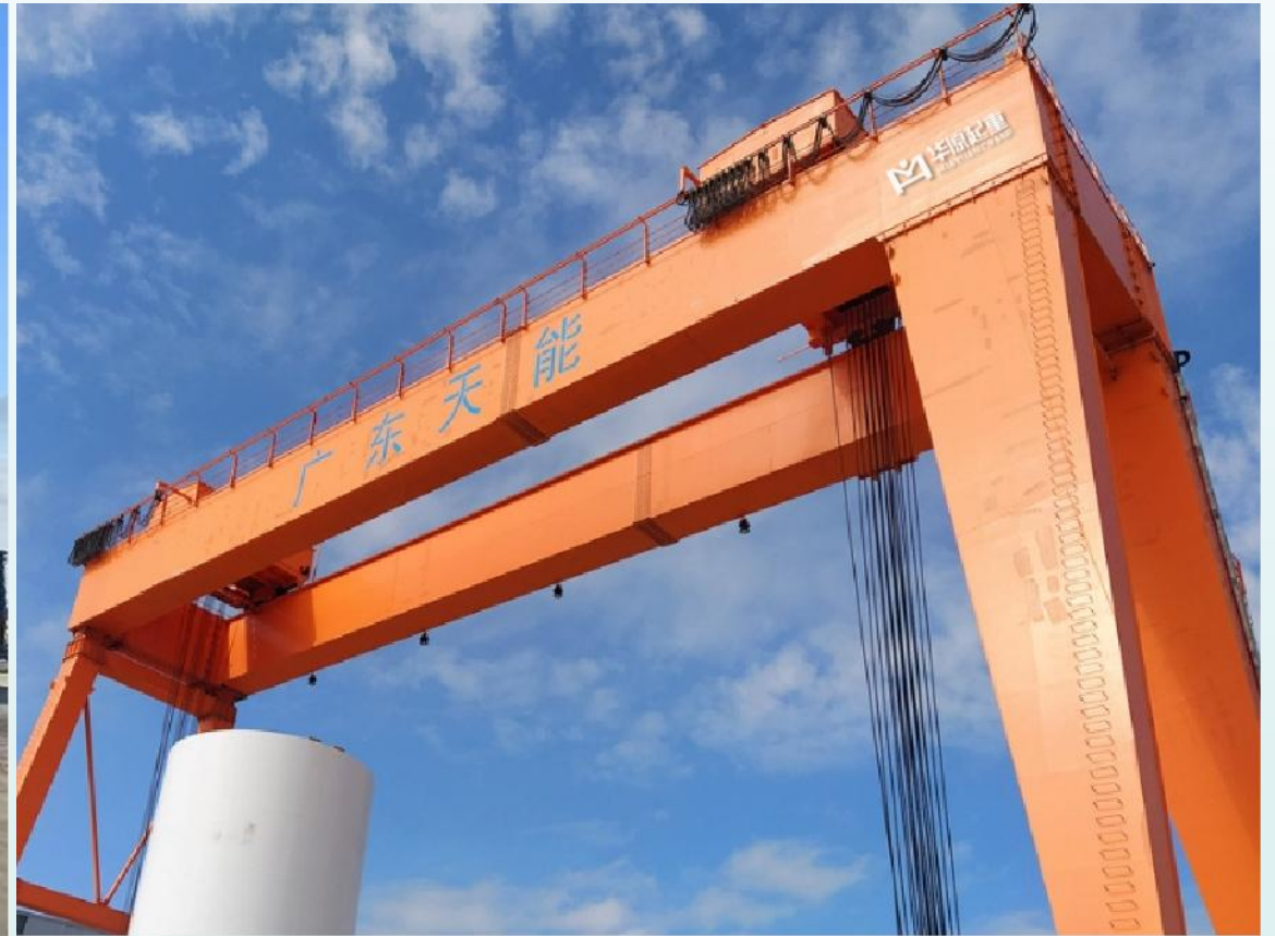
Double beam crane
